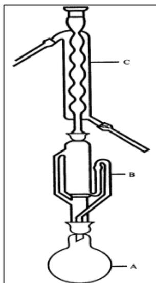
**Figura 1.** Aparato extractor Soxhlet.
