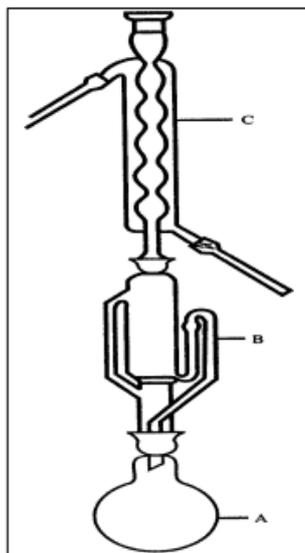
**Figura 1.** Aparelho extrator Soxhlet.
